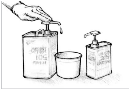
Figure 9-4 Dispense the proper proportions of resin and hardener.
