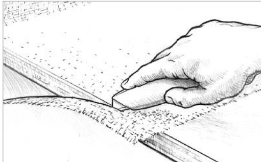
Figure 9-19 Trim excess cloth after the epoxy has begun to gel using a sharp utility knife.
