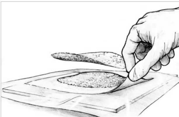
Figure 4-7 Build up a plug of wet-out fabric approximately the size, shape and depth of the hole.
