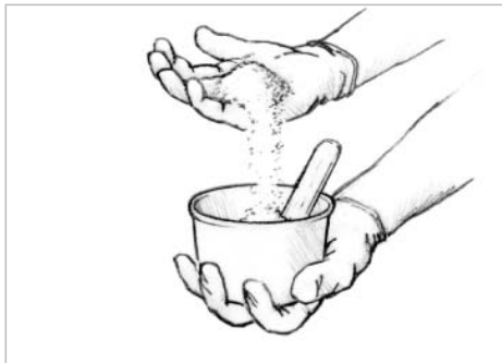
Figure 9-7 Blend in small handfuls or scoops of the appropriate filler until the desired consistency is reached.
