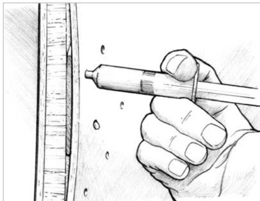
Figure 5-1 Inject epoxy under the skin using an 807 syringe with the tip cut off to match the hole diameter.
