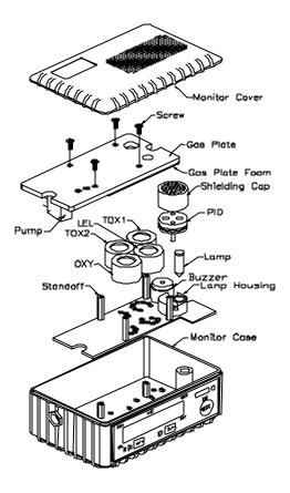
Figure 7-2 Sensor Assembly of MultiRAE PLUS
