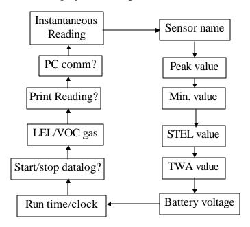
To choose a specific display, press the **[MODE]** key one or more times until the desired display appears.
