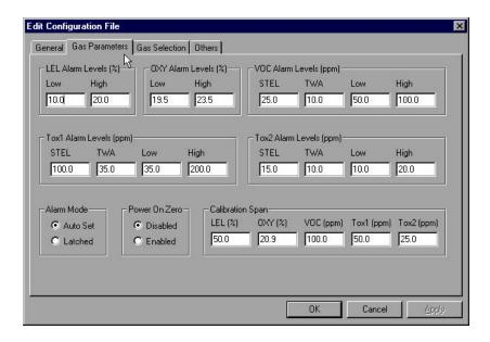
Figure 5-8 Gas Parameters Settings Tab Page **LEL Alarm Levels (%):**
