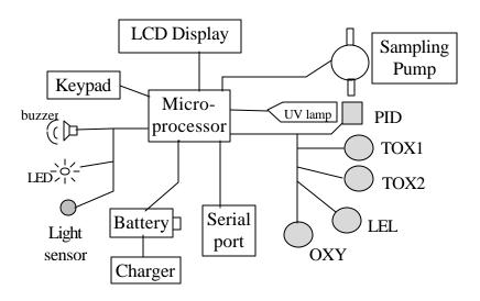
Figure 6-1 Block Diagram of MultiRAE PLUS Monitor
