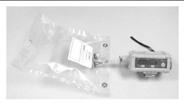
Figure 4-1 Connection of Calibration Gas
