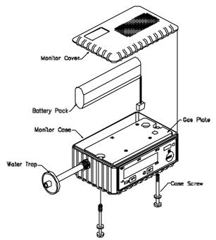
Figure 7-1 Main Components of MultiRAE PLUS
