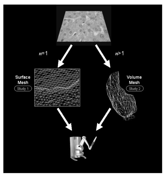
Fig. 1: Information transfer is identical for both studies: for each of the two studies pictoral information is translated into a virtual mesh to be further processed by a haptic device. The term n represents the number of digital images required for translation
