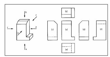
*Fig 8: Third-angle projection (DIN ISO 128-30, Figure B.1)*<sup>6</sup>
