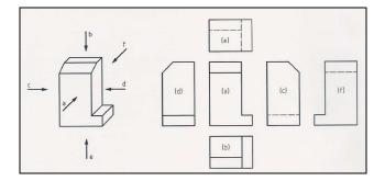
*Fig. 6: First-angle projection (DIN ISO 128-30, Figure A.1)*<sup>4</sup>
