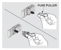
4. Check the smaller fuses by pulling out the fuse with the fuse puller provided in the interior fuse box.
