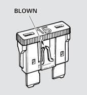
5. Look for a burned wire inside the fuse. If it is burned, replace it with one of the spare fuses of the same rating or lower.
