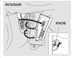
The interior fuse box is underneath the dashboard on the driver's side. To open it, turn the knob as shown.
