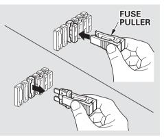
4. Check the smaller fuses in the under-hood fuse box and all the fuses in the interior fuse box by pulling out each fuse with the fuse puller provided in the door of the interior fuse box.
