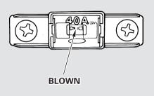
3. Check each of the large fuses in the under-hood fuse box by looking through the top at the wire inside. Removing these fuses requires a Phillips-head screwdriver.
