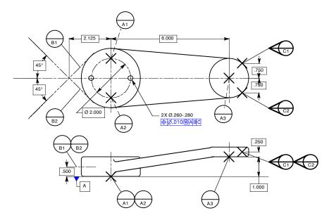
Figure 4-8 Movable Datum targets equalizing datum features
