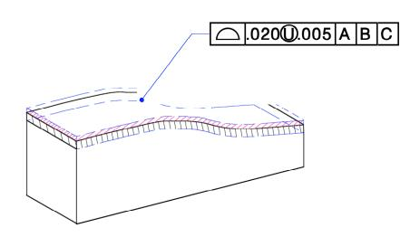
Figure 3-6 Unequally disposed profile symbol
