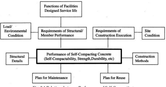
Fig. 2.1 Relations between Performance of Self-Compacting Concrete and Others
