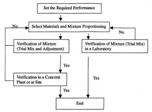
Fig.4.1 Flow Chart of Mixture Proportioning
