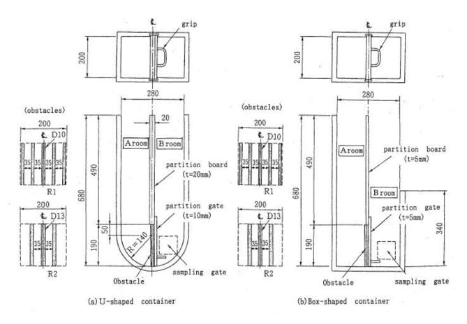
Fig.5. 1 Shapes and Dimensions of Apparatus for Self-Compactability Test
