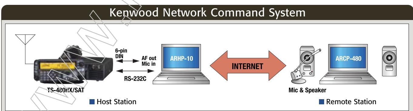
Using the ARHP-10 radio host program\*, you can even control the transceiver remotely over a LAN or via the Internet. The Kenwood Network Command System further enables VoIP (Voice over Internet Protocol) applications.
