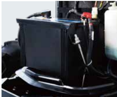
Large-capacity maintenance-free battery Gives you the power to get your working day started. Consult the battery indicators for any necessary maintenance.
