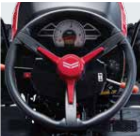
D Fully hydraulic power steering Even heavy going muddy paddies are no problem with hydraulic power steering driving you through the toughest turns.
