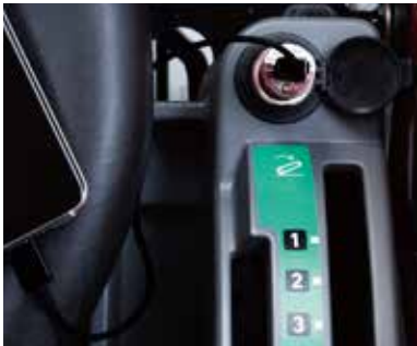
12 V accessory socket Charge smartphones and other devices while on the go. (Cigar USB Socket not included)
