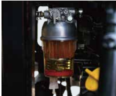
Large fuel / water separator Prevents water/moisture and dust from entering the engine.
