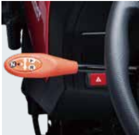
A Synchronized reverser lever Change direction, simply by shifting the lever conveniently located by the steering wheel, to back out of tight corners.
