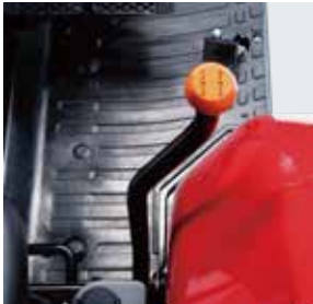
B 4 speed synchronized main shift lever Select the best speed for the job by combining the smooth changing synchronized main shift with the 2 speed range shift.
