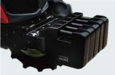
Front weight (1A8253-10300) Front bracket (1A8253-10200) Mount up to five 30kg weights for added stability.
