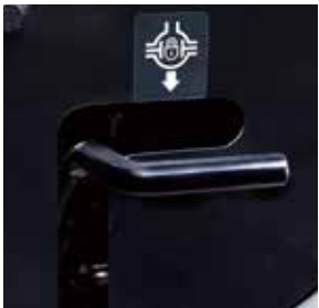
G Differential lock pedal The pedal locks the differential to keep both wheels moving and help you get through difficult paddies.
