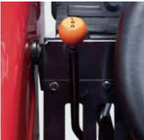
H 2 speed range shift lever The 2 speed range shift can switch between high and low speeds for use in a wide range of applications from tilling in paddy fields to traveling between fields.
