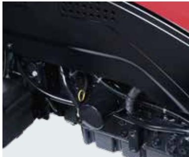
Engine oil / engine oil filter Well accessible without removing any surrounding parts like side covers. Assisting easy inspection of engine oil.
