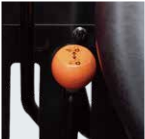
I Four-wheel drive lever A simple lever lets you switch between two and four-wheel drive for greater traction.
