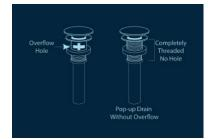
drain hole. The drain and the metal of the sink will be touching with a thin layer of plumbers putty creating a water tight seal around the drain. Wipe off excess plumbers putty, it could stain your copper sink.
