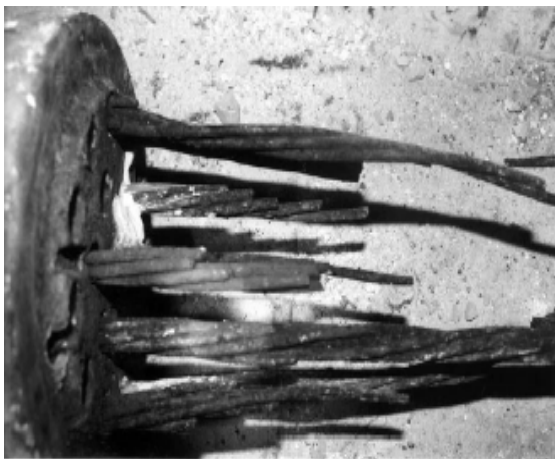
FIGURE 2 Severe Failure of Post-Tensioning Tendons near Cap Region (Corven, 2001) a) Failed tendon at Niles Channel Bridge b) Failed tendon at Column 133 NB of Sunshine Skyway Bridge
