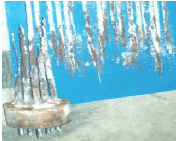
FIGURE 2 Severe Failure of Post-Tensioning Tendons near Cap Region (Corven, 2001) a) Failed tendon at Niles Channel Bridge b) Failed tendon at Column 133 NB of Sunshine Skyway Bridge
