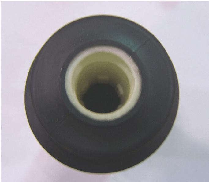
3. Glue the bumper to the inside of the dust boot (shield) as shown. Use \*3M™ Duramix™ Super Fast Adhesive, P/N 04747. Allow to cure thoroughly 5-10 minutes at room temperature.
