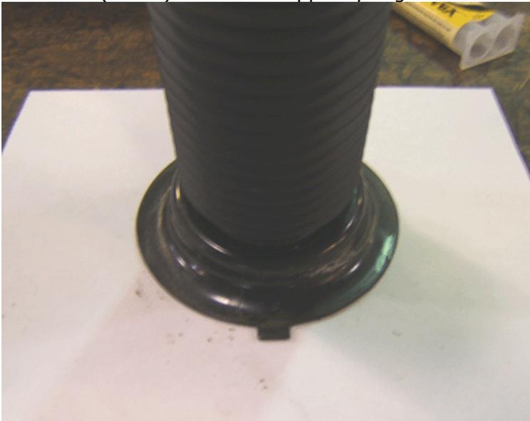
5. Glue the dust boot (shield) to the upper spring seat as shown using the above recommended adhesive. Allow to cure thoroughly.
