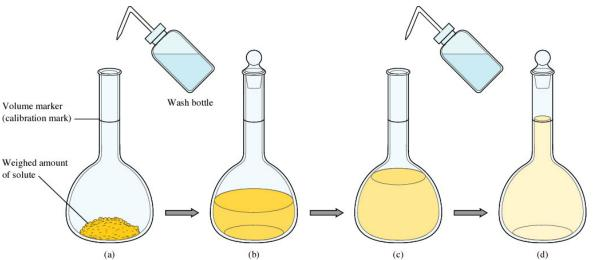
Steps involved in the preparation of a standard solution. a) A weighed amount of a substance (the solute) is put into the volumetric flask, and a small quantity of water is added. (b) The solid is dissolved in the water by gently swirling the flask (with the stopper in place). (c) More water is added, until the level of the solution just reaches the mark etched on the neck of the flask (d).
