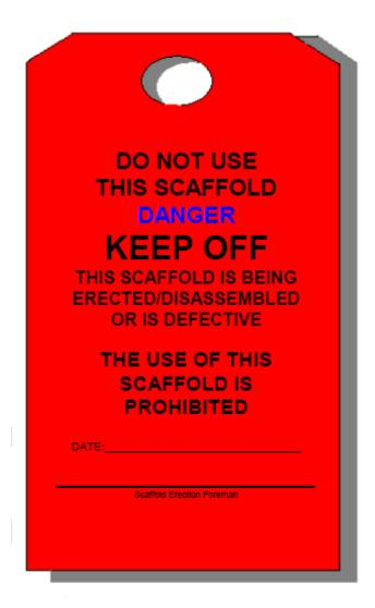
This tag must be attached to a scaffold which is partially erected or dismantled, or which is found to be defective or damaged in any way. Employees are prohibited from using this scaffold for any reason when this tag is displayed. Only authorized employees assigned to erect, dismantle, or make repairs to this scaffold are allowed on this scaffold. Authorized employees shall be required to wear and use all required personal protective equipment.
