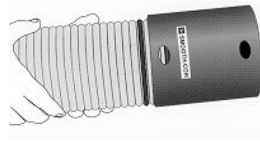
Figure 26 Key-Lock™ Couplers Insertion
