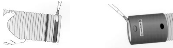
Figure 25 Key-Lock™ Couplers Lubricant Application
