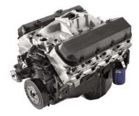
A10029 - ZZ454 Aluminum Cylinder Head 440 hp @ 5500 RPM - 500 lb-ft @ 3250 RPM 9.6:1 Compression ratio, Aluminum cylinder heads, 510/540 Hydraulic roller camshaft, 2.19 intake valve, 1.88 exhaust valve, Forged crankshaft, connecting rods, pistons, 4 bolt main block, Intake, Marine Bi-directional Waterpump, Dampner and
