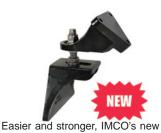
complete motor mounting system is fully adjustable (height and width) for 25" to 30" stringers. Compact size allows easy access to hoses, oil coolers, water pumps, wiring and other hardware. All parts prefabricated and ready to mount. Adjusting hardware is all stainless steel. Block mounts and stringer mounts are A-356 aluminum heattreated to T-6 full hard for maximum strength.
