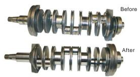
All Outboard crankshafts and wrist pins that we polish are measured, inspected and cleaned before polishing. Once polished they get a coat of rust preventative prior to shipment. Shown above is, before polishing and after.
