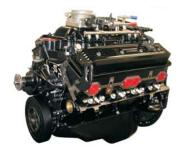
5.7 Litre 350 CID 295 hp @ 5000 RPM (PFI) 355 lb-ft @ 3600 RPM IAFM with Port Fuel Injection Vortec cylinder heads, Hyd. roller cam
