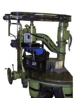
**Inboard Block & Cylinder Head Decking**
