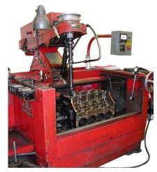
**Inboard Engine Block Honing**
