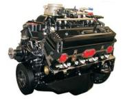
5.0 Litre 305 CID 250 hp @ 5000 RPM (PFI) 305 lb-ft @ 3500 RPM IAFM with Port Fuel Injection Vortec cylinder heads, Hyd. roller cam
