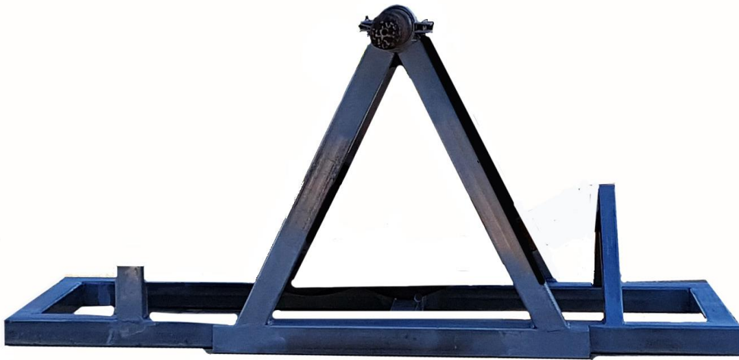
Finished frame ready to match with the nozzle housing
