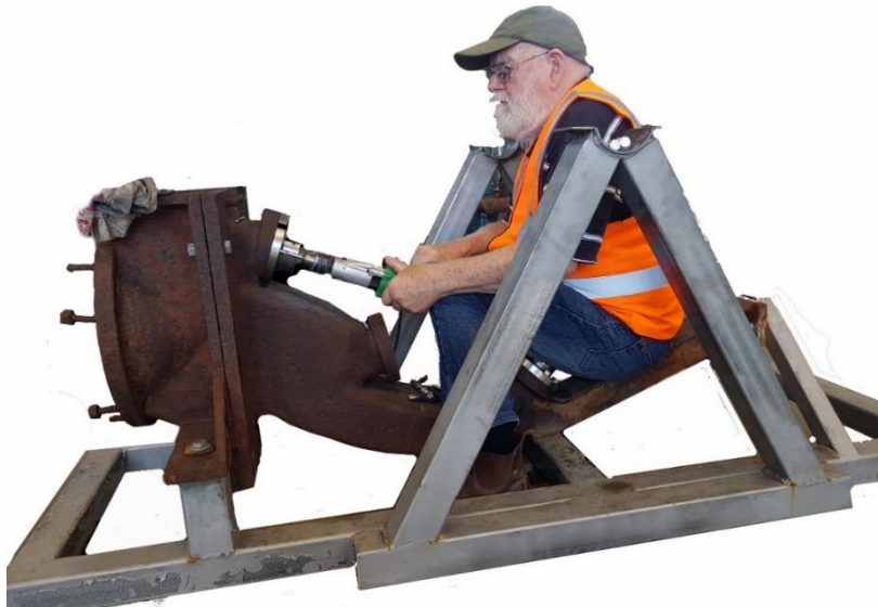
Fitting the nozzles to the nozzle housing
