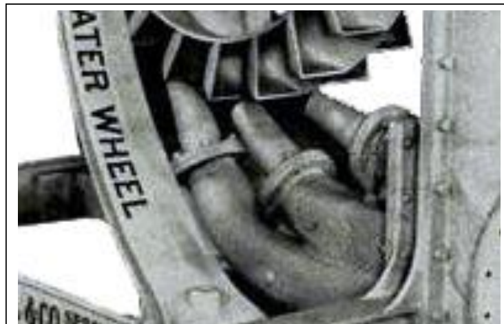
A close-up photo of the three nozzle arrangement used by the Lefell Company in one of their 1890 models. (Bob Bird collection)
