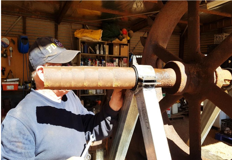
Fitting and adjusting the non-original main bearings
