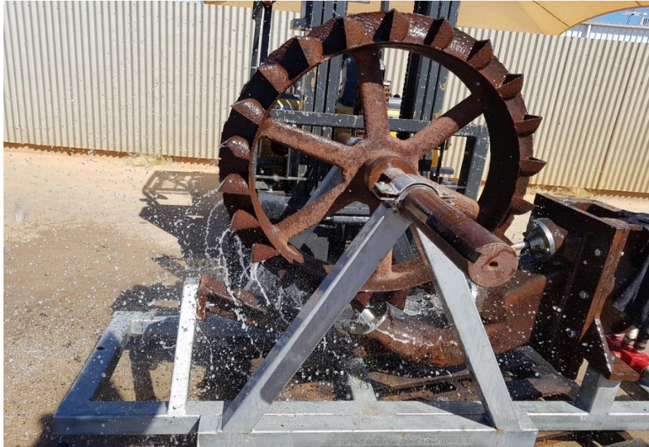
Initial start-up with the wheel assembly still on a forklift Note: In this photo, the wheel is making its first revolutions for the first time in many years. Using water pressure from a portable fire-fighting water pump. Note the input hose on the right-hand side of the photo (red) with unguarded water coming off the wheel
