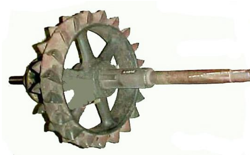
A genuine Pelton Wheel held by the Queensland Museum, showing offset buckets This patented wheel is to be found in other turbine engines (Courtesy Queensland Museum)
