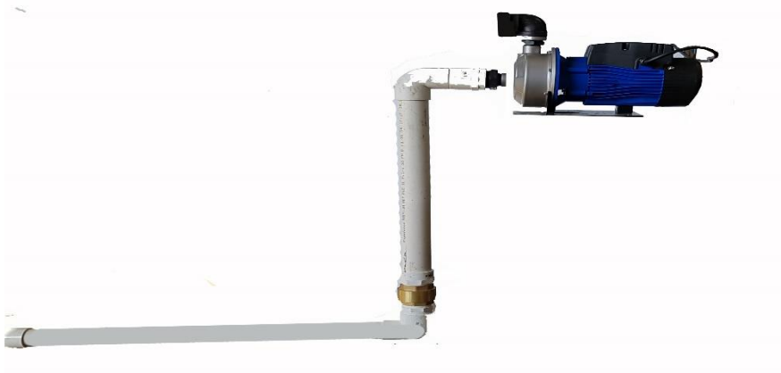
Pump assembly showing horizontal perforated water pick-up pipe (See page 16)
