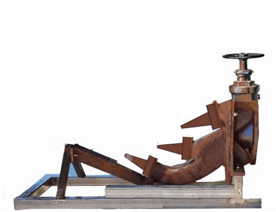
A computer image showing the gate valve, nozzles and their shrouds in place (Ian Itter collection)
