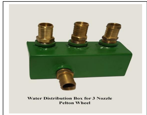
Locally manufactured water manifold showing one intake connection to a water supply hose and pump at the bottom, and three outlet fittings to connect with a \frac{3}{4} " hose connected to each nozzle
