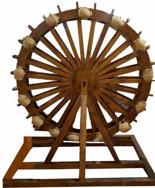
A wooden reconstructed Norian Waterwheel from the year 512AD (Courtesy Cobb and Co Museum, Toowoomba)
