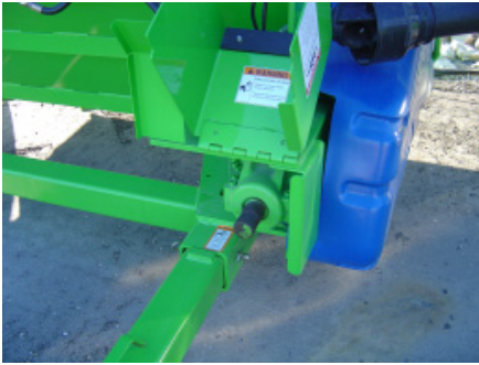
Gear Box Shaft Guard In Raised Position
