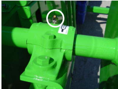
Inner Cable Drum Shaft Bearing Grease Fittings
