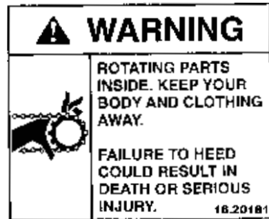
16.20181 Warning (Located on side of upper conveyor deflector)
