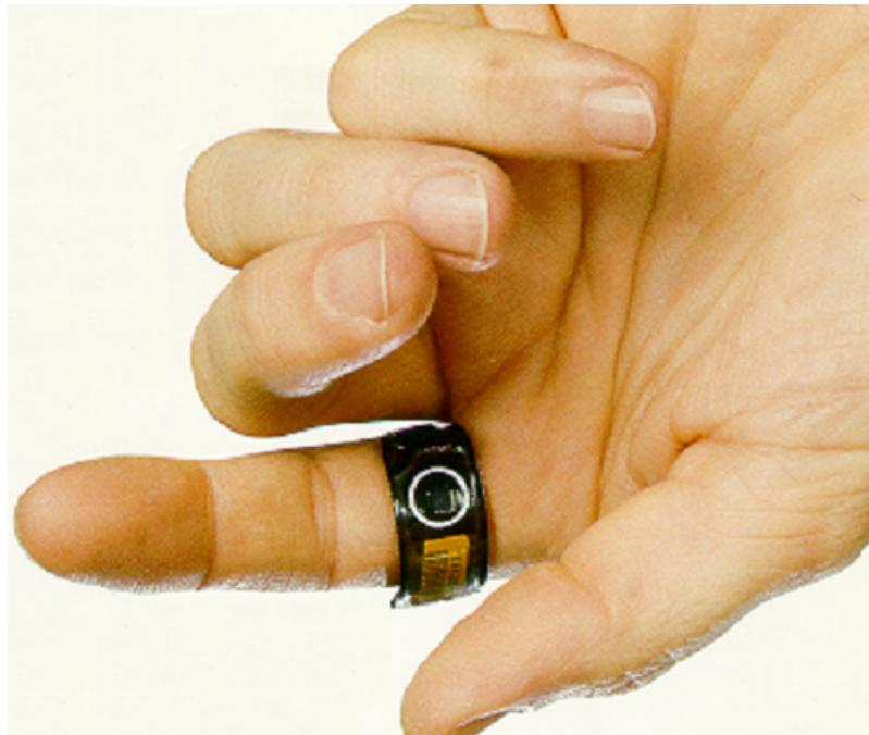
The flat portion of the ring (which contains the TLD) must be worn facing the palm or back of the dominant hand, whichever orientation will measure the greatest dose.
