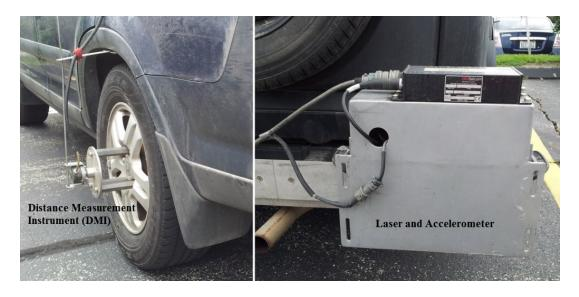
Figure 2.2 Automated pavement profiler and equipment on a typical data collection van
