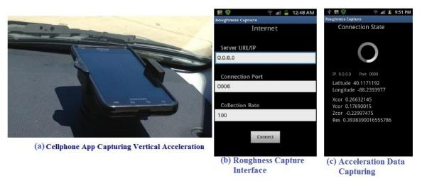
Figure 3.1 Illustration of smartphone based roughness capture system
