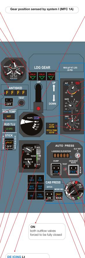
a) Illuminates when airframe deicing syst is ON. b) Flashes when airframe deicing syst still selected ON 5 min after last ice accretion detection
