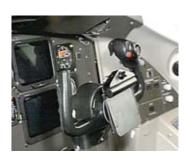
In case of jamming, pitch control will be recovered by disengaging the pitch coupling system (by applying a differential force of 52 daN).
