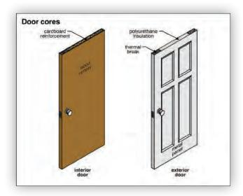
experienced when a storm door is added to an insulated metal door. The space between the doors can become overheated, and the plastic moldings may deform. In the worst cases, the metal door panel may even buckle. Many manufacturers recommend against the use of storm doors with insulated core metal doors.
