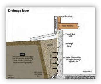
flows quickly down through it to the drainage tile.
