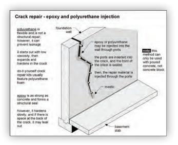
caused the crack are still present, a new crack may develop. For this reason, some contractors prefer polyurethane injection, as it stays flexible.
