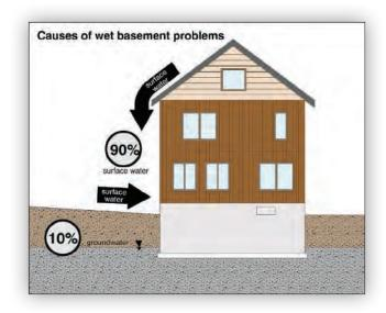
SOLVE PROBLEM Rather than trying to make a basement or crawl space into a perfectly watertight vessel, it AT THE SOURCE makes sense to keep water away from the building. It's difficult and expensive to turn a house basement into a boat. Even houses with leaky foundation walls will be dry if the water from rain and melting snow flows away from the house and does not accumulate in the soil around the building.
