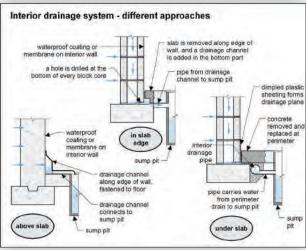
This approach is somewhat less desirable than the exterior approach, since water leaks through the exterior walls before it is carried away by this interior drainage system. The water, of course, must pass through the foundation or footing system, or go under the footing to reach this pipe. In some cases, holes are drilled through the foundation wall just above the footing to allow water to drain into this perimeter footing drain.
