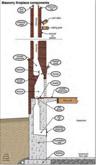
DAMPERS Masonry fireplaces have a metal damper that is usually just above the firebox. The damper may be operated from a handle on the mantle face, or a lever located inside the firebox. Dampers are closed when the fireplace is not in use to minimize heat loss. Dampers must be open for fireplaces to operate.
