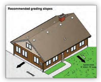
holes in foundation walls can be addressed, if needed. Large scale digging, dampproofing, drainage membranes and drainage tiles are a last resort after improving gutters and downspouts to control roof water, improving grading to drain surface water away, and correcting obvious points of water penetration.
