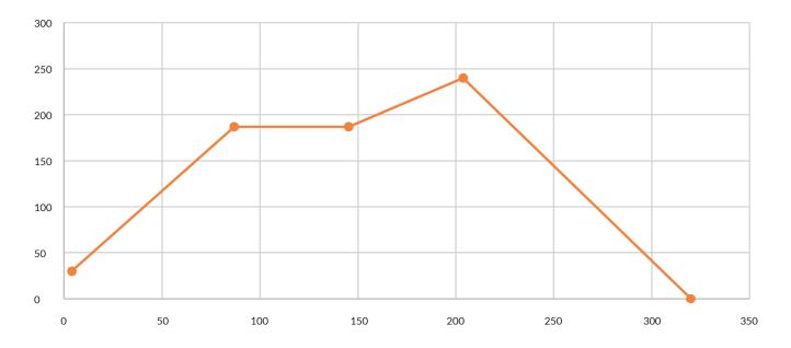
Figure 9 – Reflow soldering temperature profile (surface mount)
