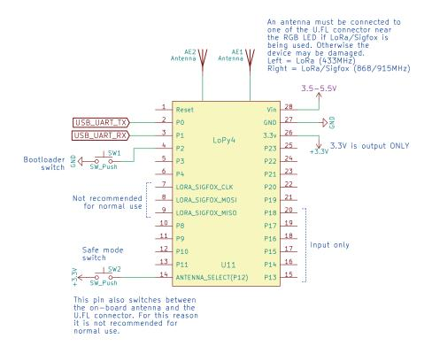
Figure 4 – Minimum required circuit
