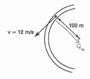
$Q_{n} = \frac{V_{n}^{2}}{V} = \frac{(12\frac{M}{s})^{2}}{100M} = 1.44\frac{M}{s^{2}}$
