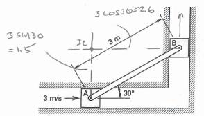
Assuming that the surfaces are frictionless, what is most nearly the velocity of block B if block A is moving at a speed of 3 m/s?
