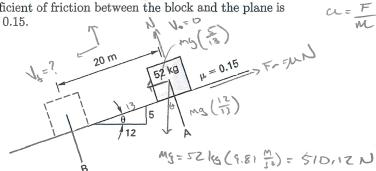
What is most nearly the velocity of the block at position B?
