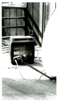
The 76 cm offset-fed dish looking at transponder 4 of SBS4, an antique satellite launched in August of 1984 and now in inclined orbit at 77°W. The 76 cm "dish-combo" comes with a .6 dB Ku-band LNBF, 60' lead-in coax and 4' of coax to go from your receiver to your TV set.
