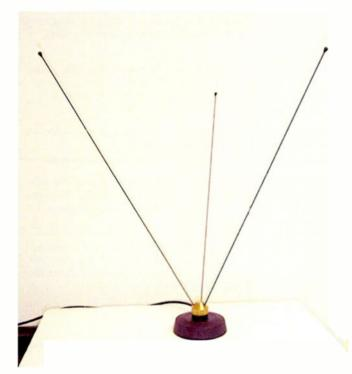
design. At higher frequencies, as an element becomes electrically longer, the radiation and reception pattern starts to favor the ends. By angling the whips downward, this pattern is also lowered toward the horizon. Now the extra length has gain over the quarter-wave whip, providing better performance. And angled downward, the antenna cluster is less likely than a comparative single vertical element to strike overhead obstacles.
