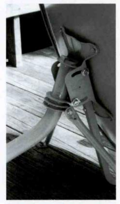
Close-up of Azimuth/Elevation mount for easy adjustment. The design of this antenna/mount is elegantly simple but well built and very easy to assemble.
