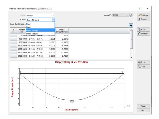
Also, the deflection criteria and the limit states calculation for the deflections with an alpha ( $\alpha$ ) angle different than zero are now done on the straight axes.
