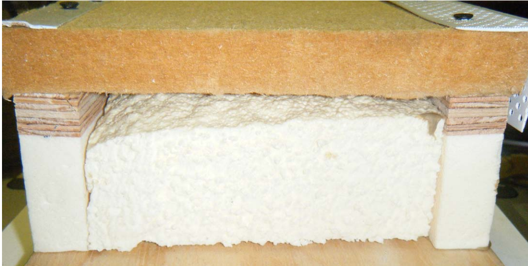
Figure 7. Mock-up of IFT insulation system: two continuous layers of insulation & air gap
