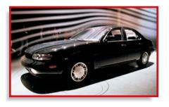
where R is the air resistance (in pounds),  $D_C$  is the drag coefficient,  $F_A$  is the frontal area of the vehicle (in square feet), and s is the speed of the vehicle (in miles per hour). The formula assumes that there is no wind.
