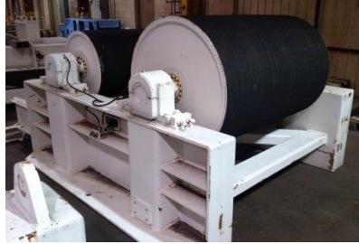
Stationery Rollers #356 26" dia 57" Face Lagged 38" dia 57" Face Lagged
