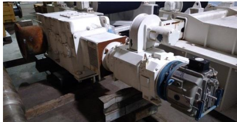
Motor & Reducer #780 100 hp 460 volt, Paramax 9000 Vao403754. 100hp Input 207:60 ratio
