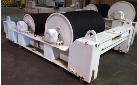
Traveling Rollers #443 26" dia 57" Face Lagged 38" dia 57" Face Lagged
