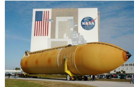
3,400 feet of weld
