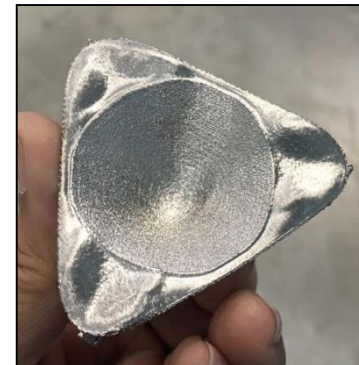
Heat build up
