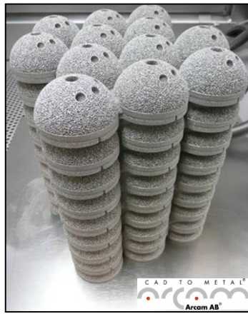
Acetabular cups with trabecular structures
