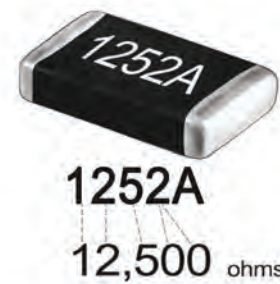
Fig. 1.16: Surface mount resistor
