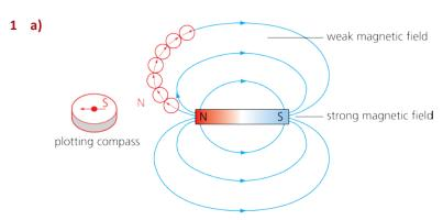
**b)** You can use the compass as shown above to trace out the pattern of field lines.
