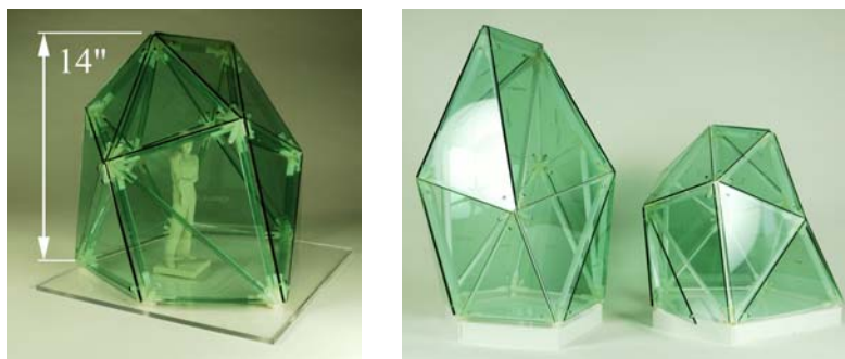
Figure 8 Final models assembled of laser cut acrylic sheets, laser cut members, FDM finger joints and glass clips printed of abs plastic.
