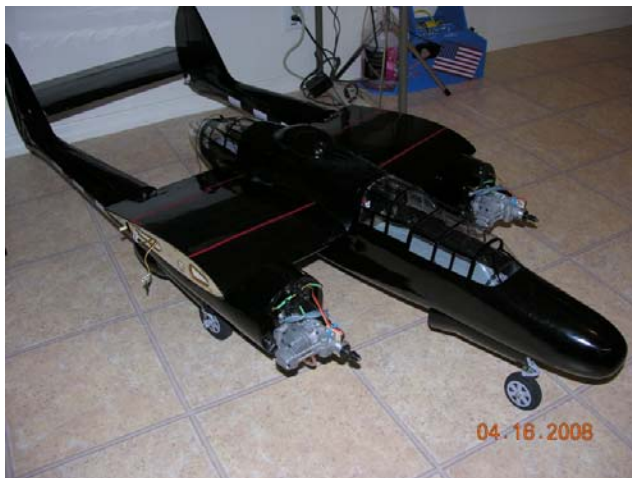
Harold Ansell's P-61 currently on the building table. It is a Advanced Scale Models ARF P-61. The wing span is 80", length is 60" and the weight is 14 pounds. The plane will be powered by twin four-stroke Magnum 52 engines. It will have 11 servos and pneumatic retracts.
