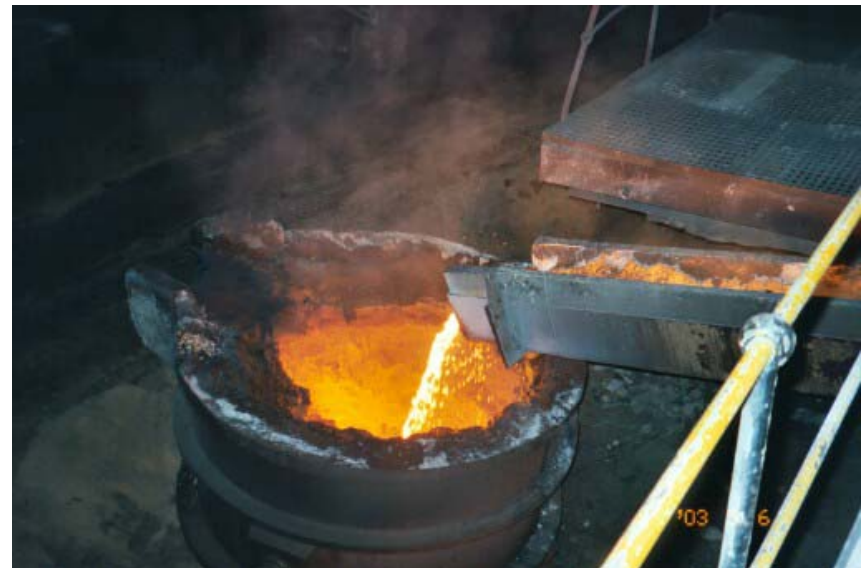
Filling a ladle to transport to the converters
