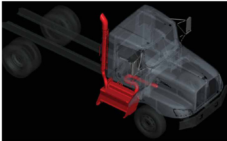
Figure 1 - Under cab DPF/SCR - Iso 1
