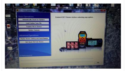
Next you need to plug your SCT into the USB port. The SCT will power up when you do this and you should have the default screen. To do this you need the cable supplied with the SCT. If you do not have one then a typical printer cable will work. The USB port will plug into the computer. Some USB ports will not work. When you have one that works you will see this
