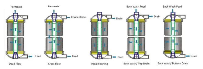
**5.2.1 Initial flushing:** The permeate valve is shut off, and an increased feed water stream is flushing the inner spaces of the membrane capillaries. This increased feed flow takes other contaminants that cannot be washed off just by water flush. This initial flushing usually takes 15-30 seconds.
