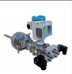
Fig. 3.1: Air purge unit LSP for automatic cleaning of pitot tubes used in gas and gas mixtures containing dust or bubbles
