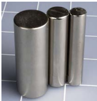
Figure 5-20. Three neodymium magnets, 1/4-, 1/2-, and 3/4-inch in diameter. I would have preferred to photograph them standing half-an-inch apart, but they refused to permit it.
