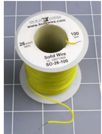
Figure 5-18. An everyday 100-foot spool of hookup wire is capable of demonstrating the inductive power of a coil.
