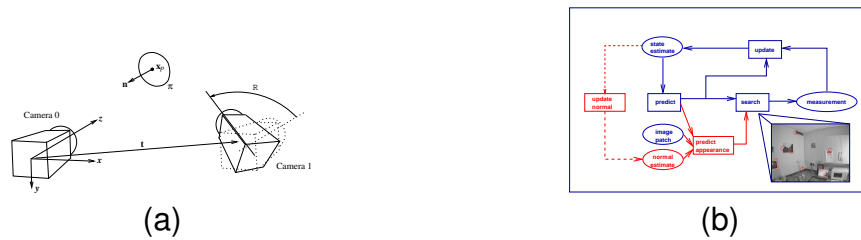
Fig. 6. (a) Geometry of a camera in two positions observing a surface with normal \mathbf{n} . (b) Processing cycle for estimating the 3D orientation of planar feature surfaces.
