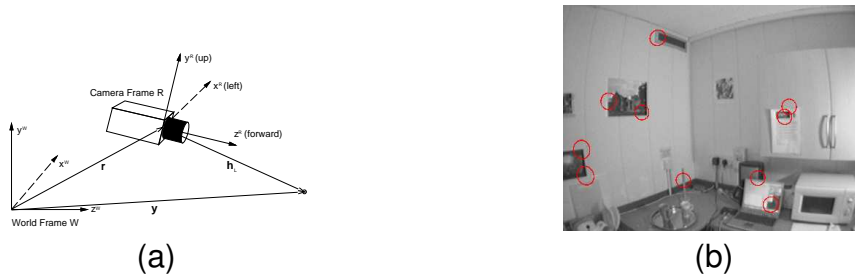
Fig. 3. (a) Frames and vectors in camera and feature geometry. (b) Active search for features in the raw images from the wide-angle camera. Ellipses show the feature search regions derived from the uncertainty in the relative positions of camera and features and only these regions are searched.
