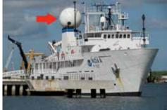
All communications with the shore are made possible by the *Okeanos Explorer's* powerful satellite dome, which enables the ship to establish high-bandwidth connectivity with Exploration Command Centers throughout the world. Image courtesy of NOAA *Okeanos Explorer* Program, INDEX-SATAL 2010 http://oceanexplorer.noaa.gov/okeanos/explorations/10index/logs/ hires/okeanos\_vsat\_hires.jpg
