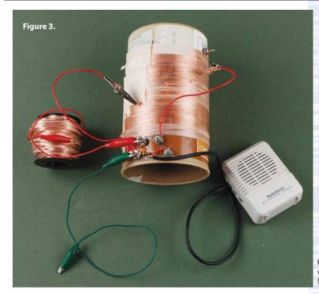
or unsafe use of ladders). You may use jumper cables for these connections as shown in Figure 3 to make it easy to disconnect your crystal set from the ground and antenna.
