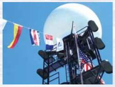
Okeanos Explorer's prominent VSAT (Very small aperture terminal) dome enables satellite communications between explorers ashore and at sea and provides multiple highdefinition video streams for widespread dissemination. Image credit: NOAA.
