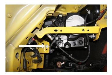
41. Working from the RH Wheel well, locate and remove the Core Support to Body Bolt
