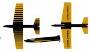
My electric powered version has a 42" span with about 325 sq, in. Power will be a Jeti Phasor 15-4 on 8 or 10 cells. It's pretty well framed out and weighs 11.5 oz. uncovered.
