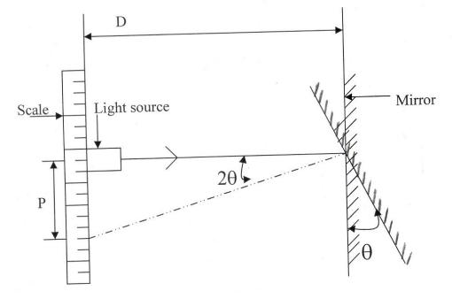
In this experiment we measure the slope at the free end of the beam using a 'Lamp, mirror and scale arrangement' (Fig. 2)
