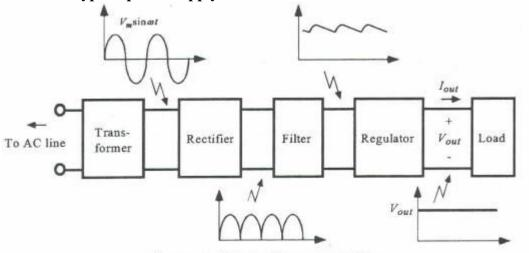
Components of a typical linear power supply
