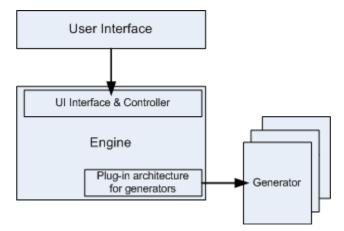
The SQL Data Generator engine defines a series of interfaces. Each interface is very lightweight.
