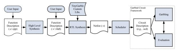
Fig. 1: Global flow of TinyGarble for both combinational and sequential synthesis. The inputs can be either a C/C++ program (translatable to HDL via a standard HLS tool) or a direct HDL description. TinyGarble is able to provide circuit description for any given GC framework.
