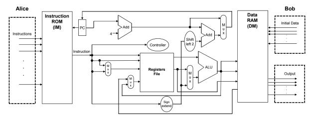
Fig. 6: Lite MIPS architecture. Alice's and Bob's inputs and the output are shown.
