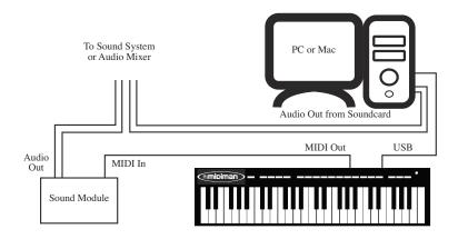
In this scenario, it may not be necessary to apply external power to the KEYSTATION. With the power switch set to "Power Off," the KEYSTATION receives power from the USB port on your computer. It is recommended that you either plug directly into the USB port on the computer, or use a powered USB hub. You may also choose to use external power form the power supply that is provided.
