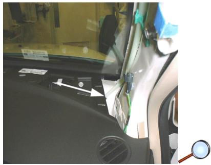
3. Remove the rubber grommet at the end of the drain tube. Refer to the illustration above.
